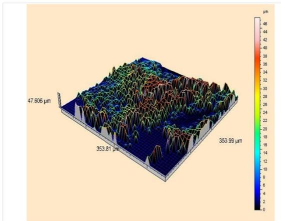
Substrate surface roughness after de-coating with abrasive blasting
