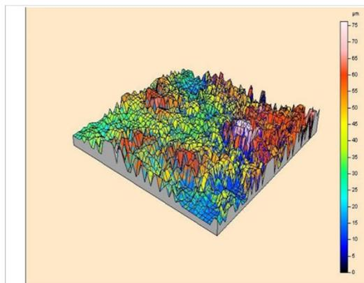
Substrate surface roughness after de-coating with water blasting
