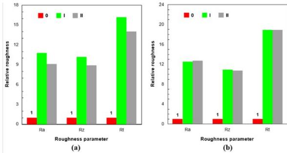
Substrate surface roughness measurements.
