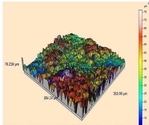
Substrate surface roughness after primary abrasive blasting
